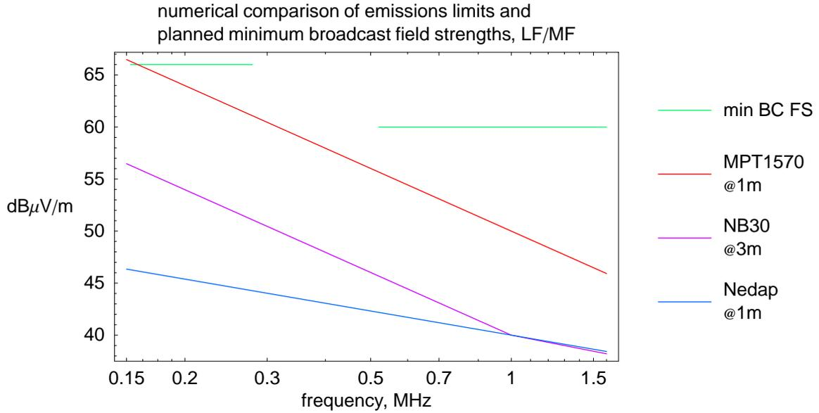
Note however that this diagram can be misleading. The NB30 limit is specified at a distance of 3 m, whereas the other two are specified at 1 m. It is customary to assume that the field falls off as  $1/r$ , whereupon a correction of  $20 \text{Log}_{10}[3] \approx 9.54 \text{ dB}$  is appropriate to convert from one distance to the other. This is done in the following graph:
