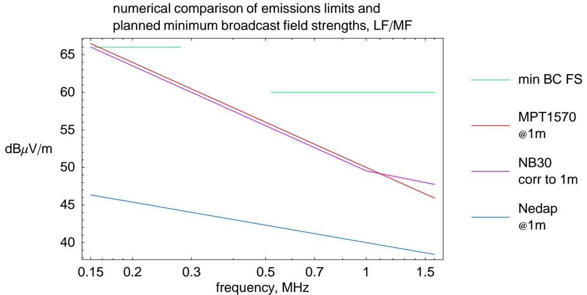
This now enables the protection given by the various limits at the distance of 1 m (representative of indoor listening) to be properly compared. It is clear that the Nedap proposal would give much greater protection than the other two — which are very similar. However in assessing the *absolute* level of protection we must also take account of the fact that all the limits specify the use of a *peak detector* when making the measurement.
